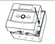
• Refit the MCP to the backbox, hooking it up from the top and pushing it towards the backbox.
