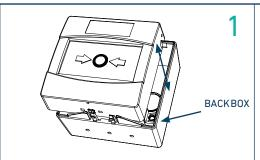
Remove the MCP front from the backbox using key provided.
